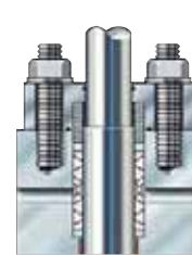
Triple seal, double PTFE cup and cone (self-adjusting/self-contained) with lantern ring. 2 in (50 mm) – 12 in (300 mm) ASME Class150 only (purge ports are an additional option)
